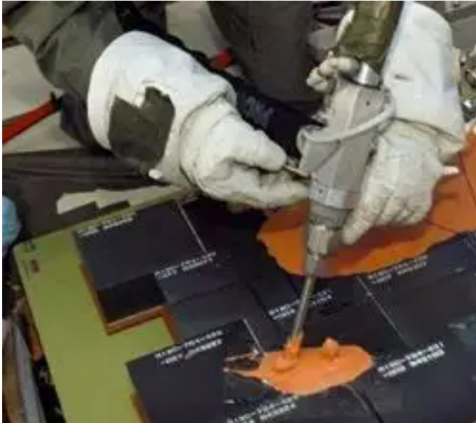
A goo gun for repairing damaged heat-resistant tiles has been tested in aircraft and will fly on Discovery. (Image&colon; NASA)
